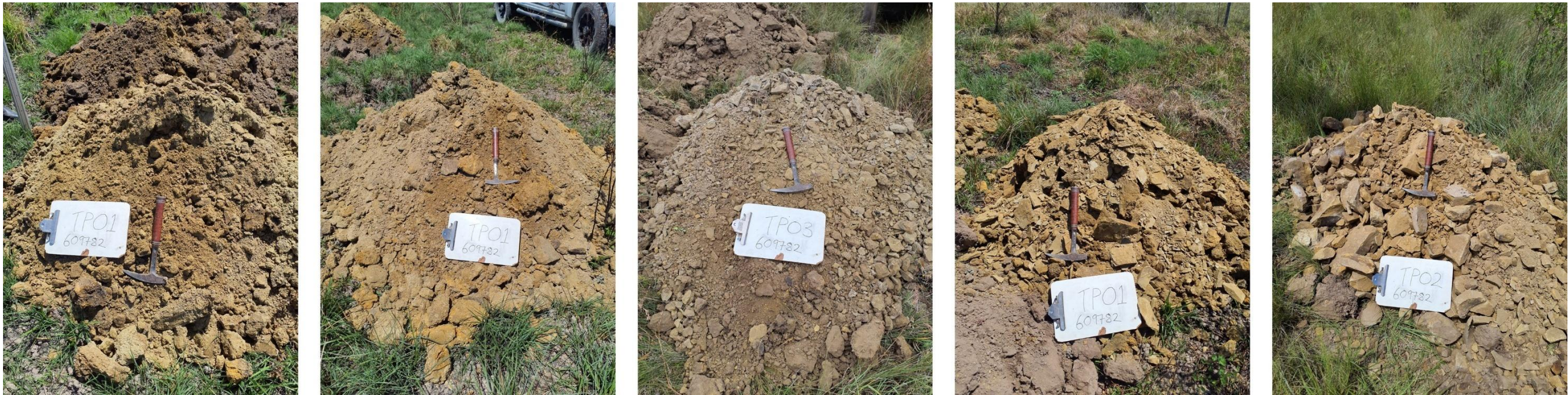
Figure 5-3: Excavated stockpiles of Layer 2 (left), Layer 4 (left centre), Layer 5 (centre), Layer 6 (right centre) and Layer 7 (right)
